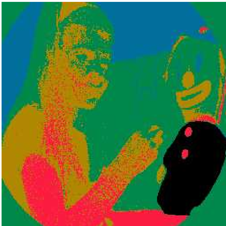
Figure 7.10: Result of segmenting the BBC testcard using Forgy's method ( k = 7 ).
