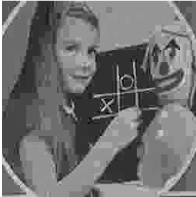
Figure 6.10: BBC testcard image reconstructed from a DCT based compression, with a compression ratio of 100:1.
