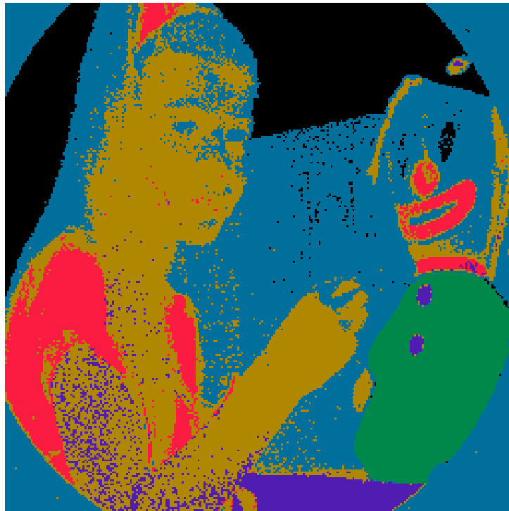
Figure 7.7: Result of segmenting the BBC testcard using Naylor's method (6 classes found).
