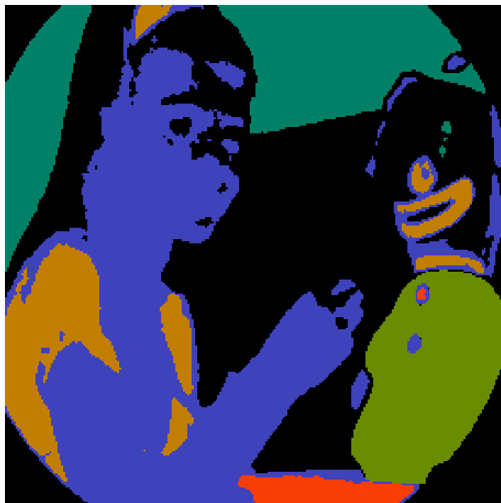
Figure 4.26: Segmentation of the colour BBC testcard image, produced with both smoothing and lighting effect removal.
